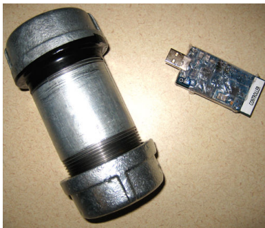
Figure 11: Our Implementation Using Galvanized Steel Pipe
