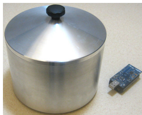
Figure 13: Bigger and Ergonomically-friendly Faraday Cage This Faraday cage may resemble a storage container for baking goods, but it is heavier, air-tight, and attenuates radio signals.
